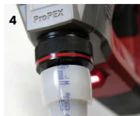
Figure 9: Expansion with Milwaukee M18 ProPEX Expansion Tool
