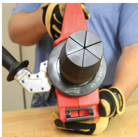
Figure 13: Correct expansion head alignment
