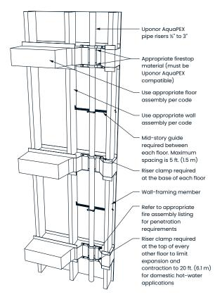
Figure 70: Domestic hot-water riser detail
