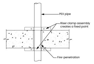
Figure 64: Fixed point example 2 (vertical)
