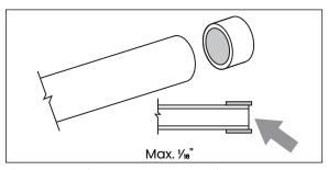
Figure 32: Slide the expanded ring over the end of the piping
