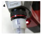
Figure 9: Expansion with Milwaukee M18
