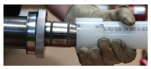
Figure 22: Slide head into piping
