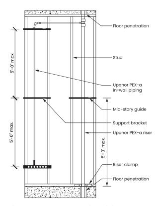
Figure 62: In-wall versus riser piping
