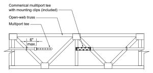
Figure 51: Supporting multiport tees on open-web wood trusses
