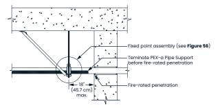
Figure 57: Fixed points near a fire-rated penetration (horizontal)
