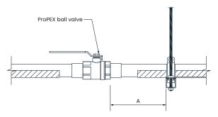
Figure 44: Supporting 11/4" to 2" ball valves
