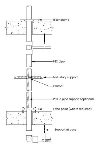
Figure 65: PEX riser detail
