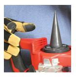
Figure 10: FORCE LOGIC expansion head installation
