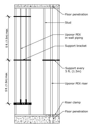
Figure 67: In-wall versus riser piping
