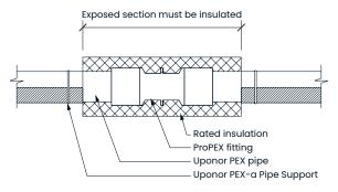
Figure 59: PEX-a Pipe Support installations in ASTM E84 applications
