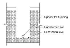
**Figure 81: Good soil conditions** — If the trench is dug smoothly, install the piping directly on the prepared bottom. The bottom must be flat with no hollows, lumps or rocks.
