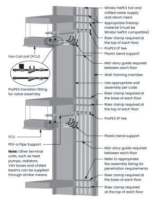
Figure 69: Hydronic piping riser detail
