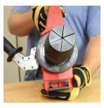
Figure 13: Correct expansion head alignment
