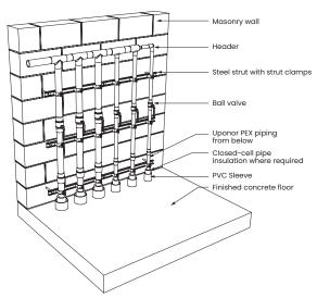
Figure 78: Mechanical room transition (below-grade piping)
