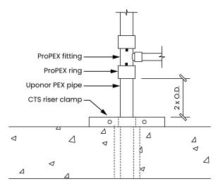
Figure 66: Clamp distance example
