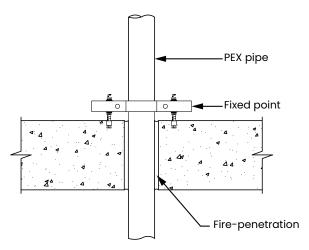
Figure 63: Fixed point example 1 (vertical)
