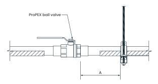
Figure 60: Supporting 1¼" to 2" ball valves
