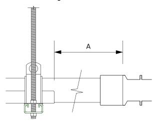
Figure 47: Minimum distance to fitting
