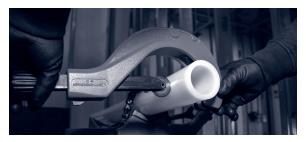
Figure 33: Uponor swing-style pipe cutter for up to 4" pipe (E6084000)
