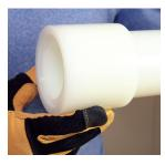
Figure 16: Ensure ring reaches stop edge
