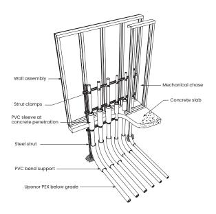
Figure 79: Wet-wall chase transition (below-grade piping)
