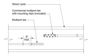
Figure 50: Supporting multiport tees on wood I-joists
