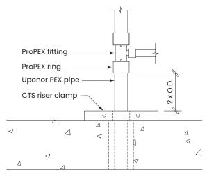
Figure 68: Riser clamp detail
