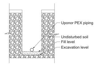
Figure 82: Poor soil conditions — With rocky, clay, muddy or other poor soil conditions, it may be necessary to prepare the trench bottom using granular material of such size and grading to provide a stable base. See local code for additional requirements.
