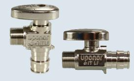
The ProPEX straight and angle stop valves feature an ASTM F1960 connection for ½" Uponor AquaPEX pipe and a ¾" male threaded connection for fixture risers.
