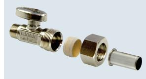
Compression straight and angle stop valves include a Teflon®coated brass compression ring and a stainless-steel insert for compression connection to ½" Uponor AquaPEX pipe and a 3%" male threaded connection for fixture risers.
