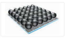
The Coolslab $^{\circ}$  system, as developed by Hanson and Uponor. The Uponor Contec system is prefabricated in the precast section
