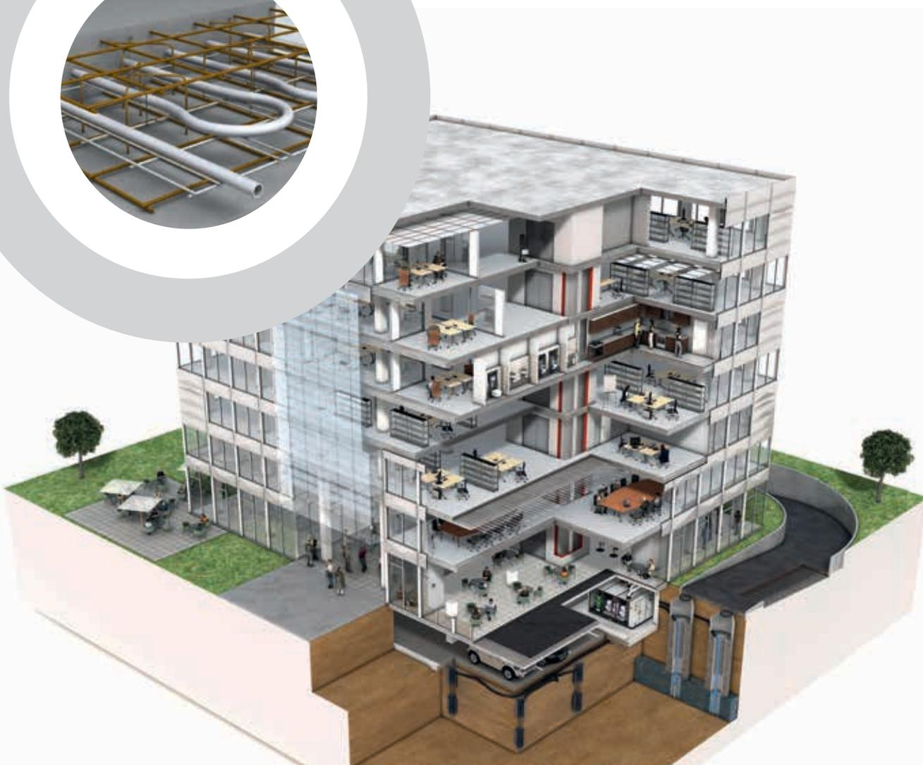
The flexibility and adaptability of the Uponor Contec system is demonstrated by the fact that it has already been installed in all possible slab or wall constructions. Whether the selected construction method is cast in situ, filigree (part precast), fully precast or permanent formwork, the Uponor Contec system is flexible enough to meet project demands in conjunction with the related variations of slab constructions.
