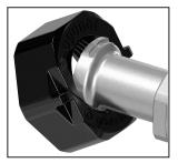
Step 2: Insert large tab into nut.
