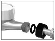
**Step 3:** Fasten assembly to meter. Hand tighten plus up to ½ turn.
