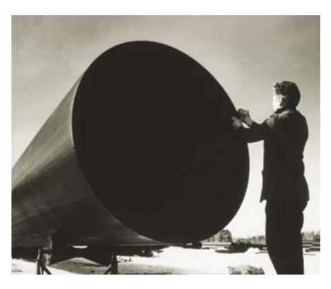
pipes produced using extrusion technology.
