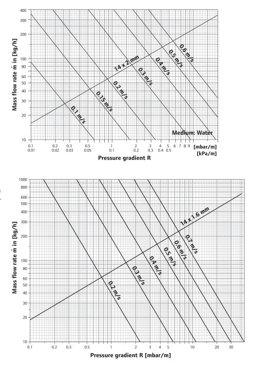
The pressure losses in the Uponor multi-layer composite pipes can be determined with the aid of the diagram
