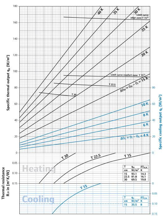
Design diagram heating/cooling for Uponor Siccus 14 x 2 mm with cement screed load distribution layer including KB 650N (s\_{u} = 30 mm with  $I_{u}$  = 0.28 W/mK)
