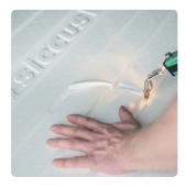
Additional channels are created using the electric cutting tool
