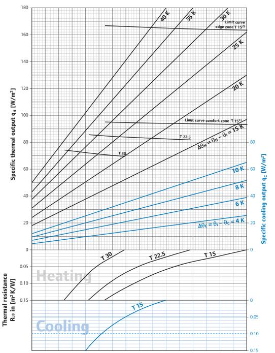
Design diagram heating/cooling for Uponor Siccus 14 x 1.6mm MLCP Pipe with cement screed load distribution layer including KB 650N
