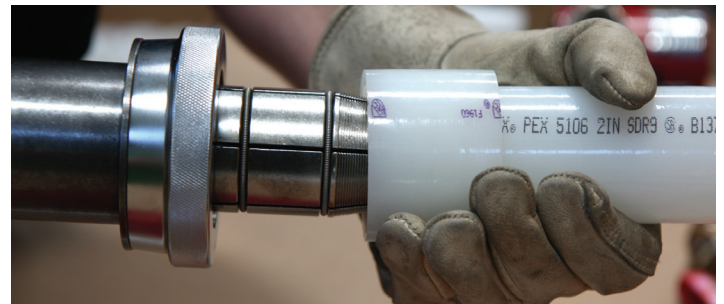
Figure 2-22: Slide head into piping
