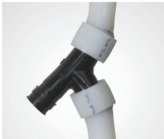
Figure 1-7: At approximately 2,900 lbs. of pull force
