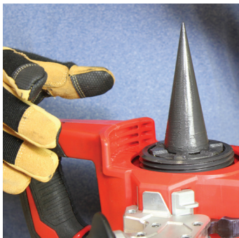
Figure 2-10: FORCE LOGIC expansion head installation
