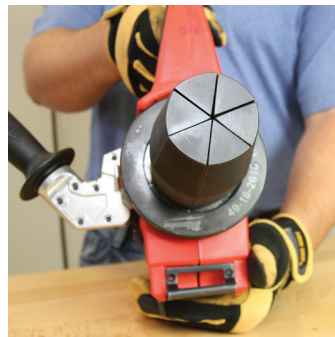
Figure 2-13: Correct expansion head alignment
