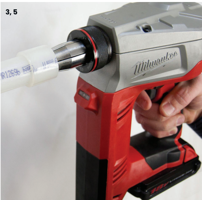
Figure 2-9: Expansion with Milwaukee M18 ProPEX Expansion Tool
