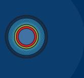
For the same heat loss as with VIP, an outer diameter of more than double the size is required.
