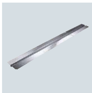
Uponor Siccus heat conducting lamellas – stable aluminium lamellas with omega groove for optimal heat transfer to the system pipe 2-fold pre-punching for simple shortening without tools of the lamella size 120 x 1180 mm.
