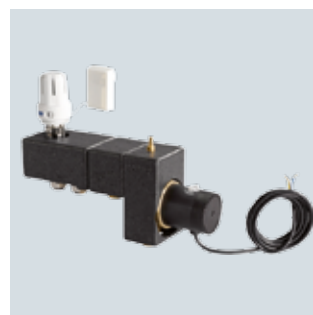
Uponor Fluvia T Push-12 mini pump groups for individual rooms and small heating surfaces. Room temperature regulation optionally via thermostat head with capillary room temperature sensor or Uponor room sensor (wire-based or wireless) with thermal drive. Ideal for connecting the radiant heating to an existing high temperature system.
