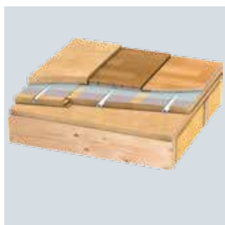
Uponor Tignum panel on wooden joist
