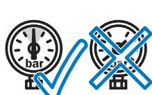
After 2 hrs. check for leakage
