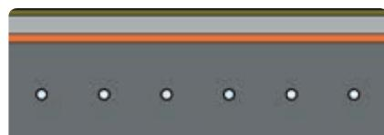
Concrete slab with impact sound insulation
