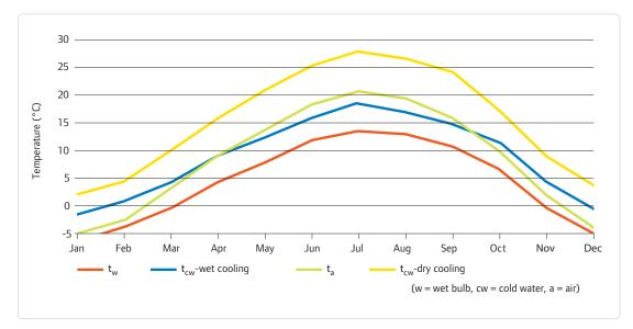
Cold water temperatures achievable with wet and dry cooling towers over the course of a year after Fackel-mayer
