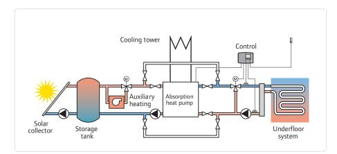
Cold water generation with solar thermal support
