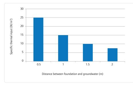
Specific thermal input (~ cooling load density) of a floor slab cooling system depending on the distance between groundwater and foundation (moist cohesive floor/saturated gravel or sand)
