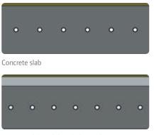
Concrete slabs with only a thin floor covering or bonded screed deliver a maximum heating or cooling capacity upwards into the room.
