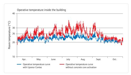
Comparison of simulated dry resultant temperature curves: In summer, concrete core activation can effectively counteract overheating of the building – apart from isolated occasions, the room temperature remains below 26 °C
