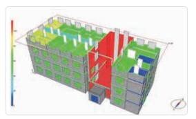
Cooling load simulation of an office building
