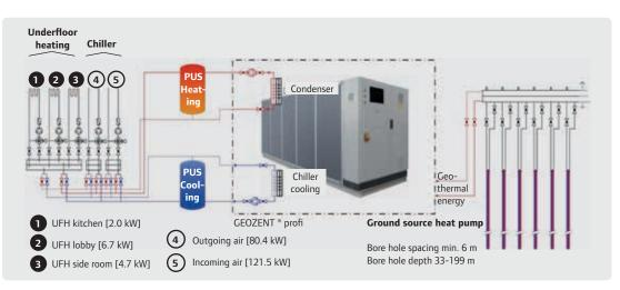
Function chart of geothermal energy supply with Geozent® profi
