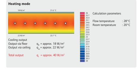
Thermal output of a concrete slab with stepsound insulation layer
