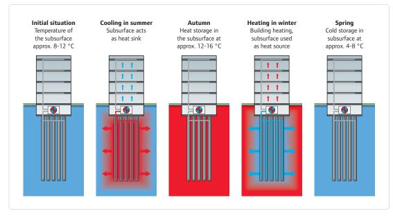
Energy piles: thermal utilisation of the subsurface
