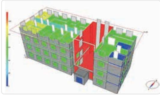
Cooling load simulation of an office building
