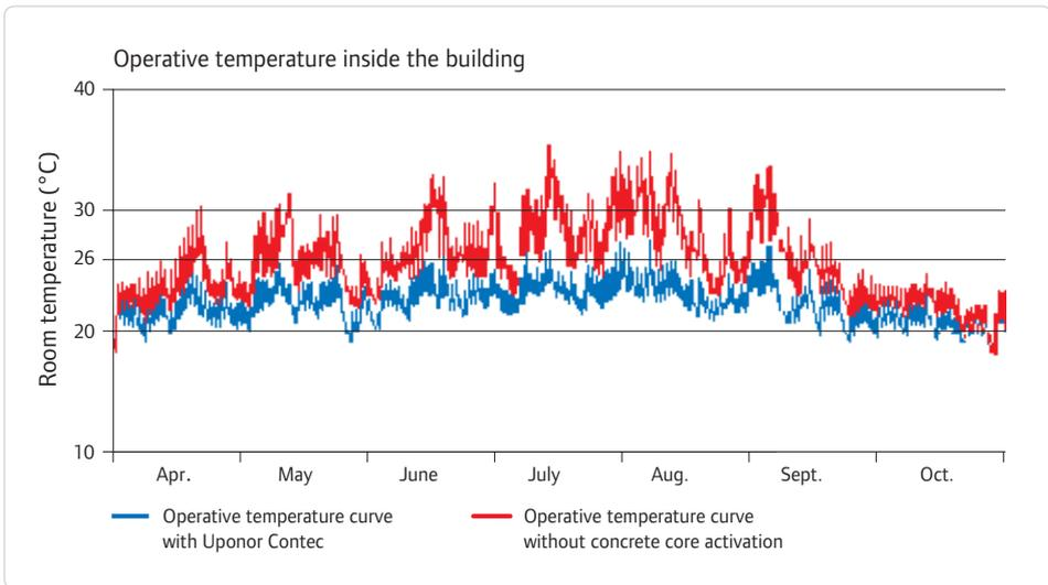
Comparison of simulated dry resultant temperature curves:
