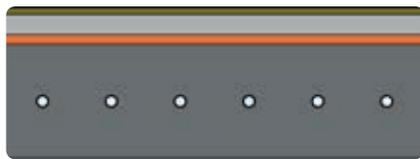
Concrete slab with impact sound insulation
