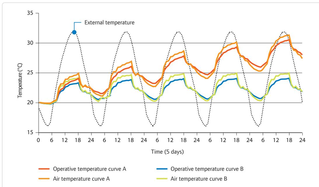
A) Due to the higher thermal mass and the smaller window area ratio, compared with the previous building this building is less sensitive to internal and exterior loads. Nevertheless, by the 5th day of the hot spell, the internal temperature has reached more than 30 °C.
