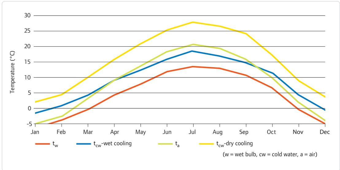
Cold water temperatures achievable with wet and dry cooling towers over the course of a year after Fackel-mayer
