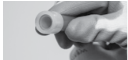
Figure 3-8: Ensure pipe reaches ring's stop edge
