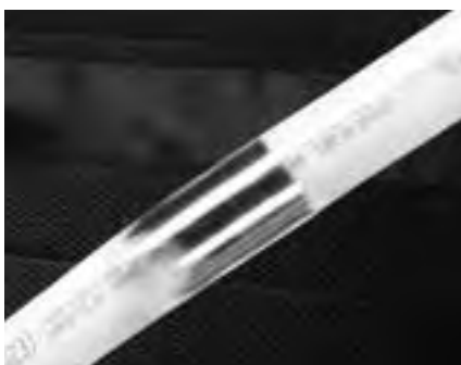
Figure C-1: Reforming kinked piping
