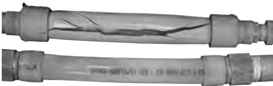
Figure C-2: CPVC vs. PEX freeze test
