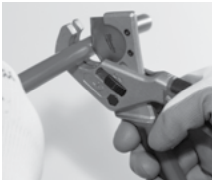
Figure 3-6: Square cut the pipe
