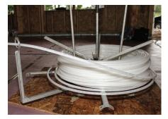
Figure 3-1: PEX Uncoiler
