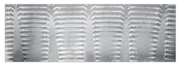
Figure 4-32: Expansion without proper rotation
