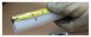
Figure 4-29: Measure from end of pipe
