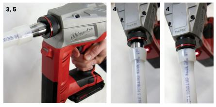
Figure 4-10: Expansion with Milwaukee M18 ProPEX Expansion Tool
