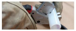
Figure 4-30: Cut pipe at marking
