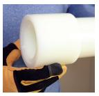
Figure 4-17: Ensure ring reaches stop edge
