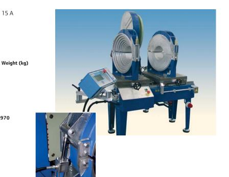
On request available with hydraulic clamping system.
