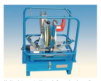
Machines being cap sizeable into the frame reduce the overall dimensions for the transport and stocking when not in use.
