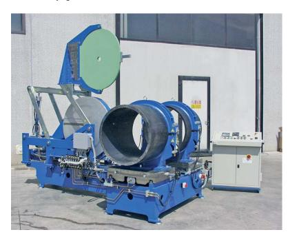
**PL 125 C and PL 160 C** are manually working workshop machines to produce high quality segmented bends in all pressure classes.
