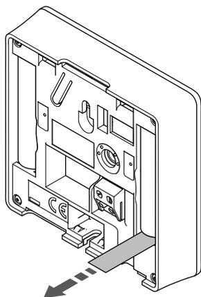
Remove the plastic transportation strips from the batteries to start the thermostat.
