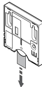
Remove the plastic transportation strip from the battery to start the thermostat.
