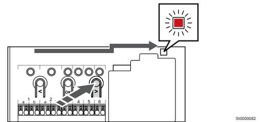
Use buttons < > to move the pointer to the power LED (LED flashes red).
