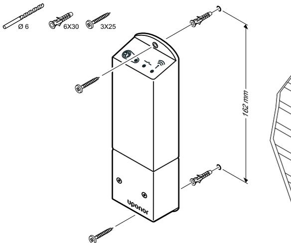
Attach the relay module to the wall using screws and wall plugs.
