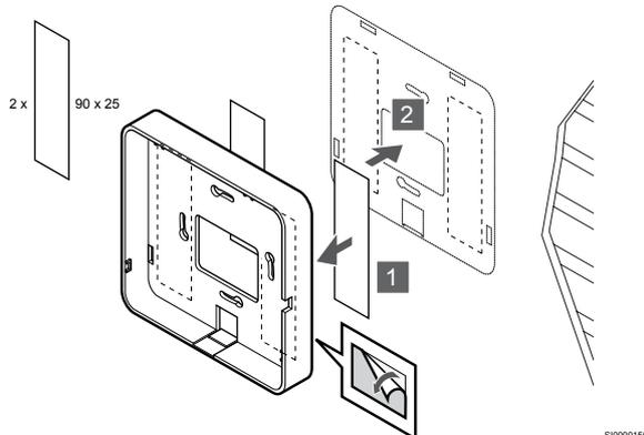
Attach the communication module back mount to the wall using adhesive tape.
