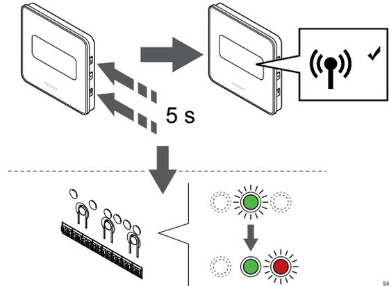
Press and hold both **▲** and **▼** buttons on the thermostat until the text **CnF** (configure) and a communication icon is displayed.
