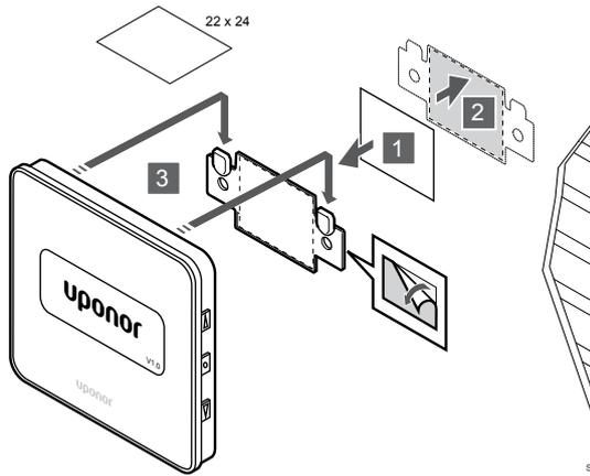
Attach the thermostat to the wall using the wall bracket and adhesive strips.
