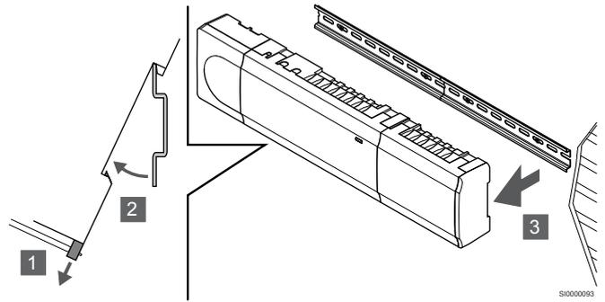
1. Use a screwdriver (or similar) and extend the springy plastic catcher from the room controller.
