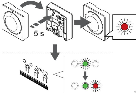
Gently press and hold the registration button on the thermostat, release when the LED on the front of the thermostat starts flashing.
