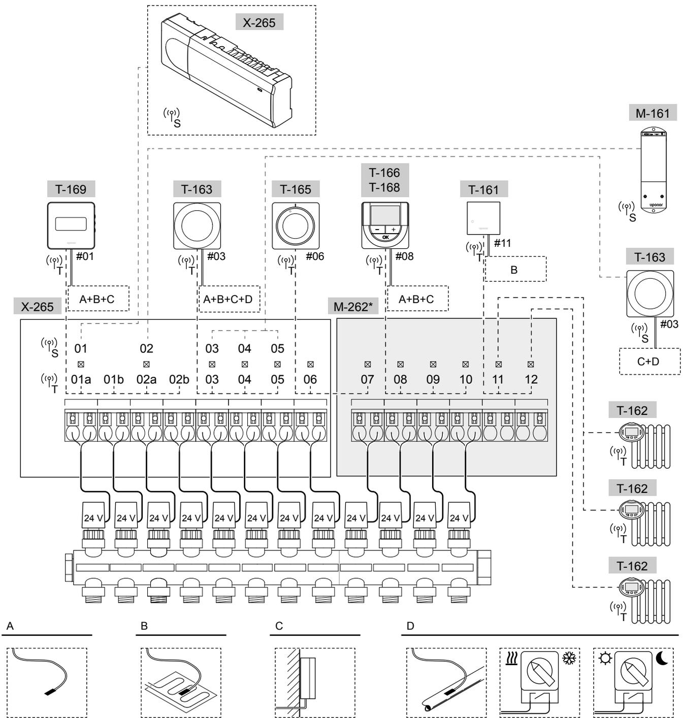
\*) This example contains optional accessories which adds six actuator outputs (slave module M-262) to the Uponor Smatrix Wave Pulse room controller
