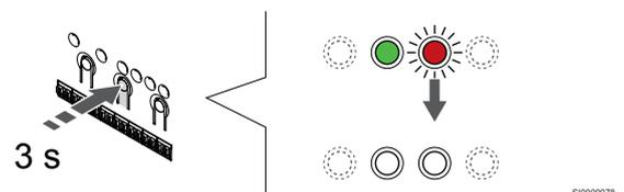
Press and hold the **OK** button on the room controller until the green LEDs turn off to end registration and return to run mode.
