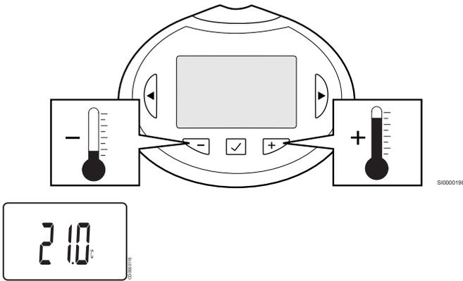
To adjust the temperature setpoint of the current control mode on the thermostatic head:
