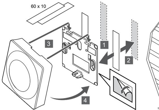
Attach the thermostat to the wall using the wall bracket and adhesive strips.
