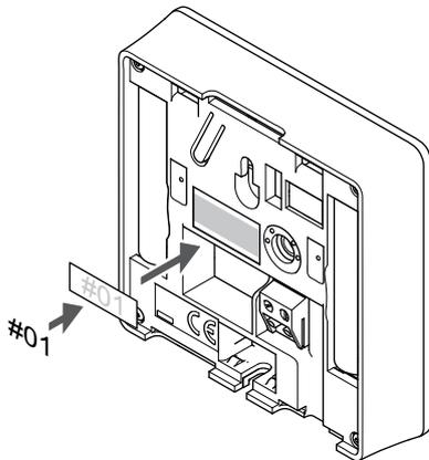
Label the thermostat, where suitable, with the channel numbers they are to control, for example, #02, #03. For a system with several room controllers, add the ID of each room controller, for example, 1.02, 1.03, 2.02, 2.03.
