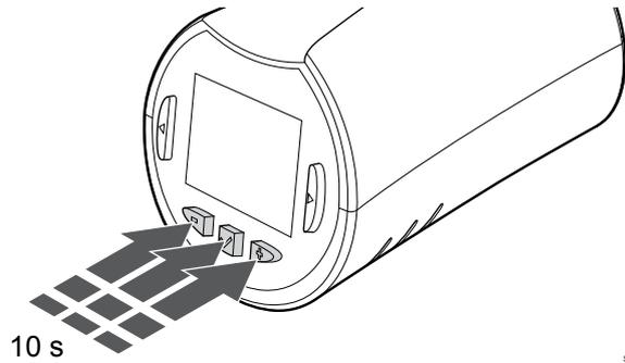
To factory reset the thermostatic head:
