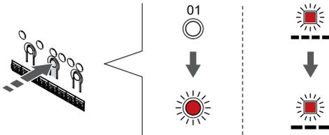
Press the **OK** button to enter system device registration mode (power LED). The power LED starts flashing according to the pattern long blink, short pause, long blink. Channel 1 starts flashing red.
