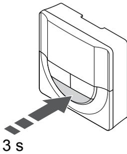
Press and hold the **OK** button for about 3 seconds to exit the settings menu.
