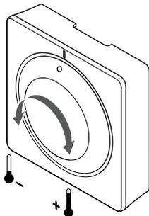
To adjust the thermostat temperature setpoint:
