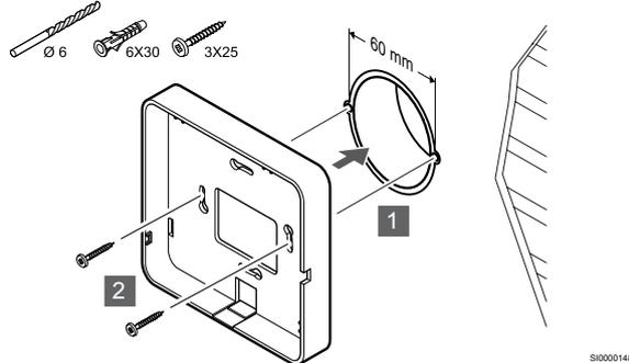
Attach the communication module back mount to the wall box.
