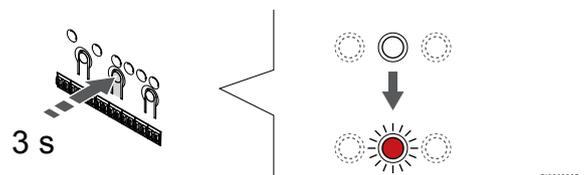
Press and hold the **OK** button on the room controller until the LED for channel 1 (or the first unregistered channel) flashes red.
