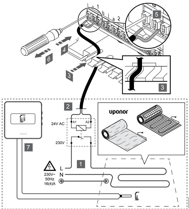
1. Connect the electrical underfloor heating mat/wire to a 24V AC relay dimensioned for the correct load.
