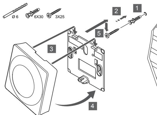
Attach the thermostat to the wall using the screw and wall plug.
