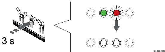
Press and hold the **OK** button on the room controller until the green LEDs turn off to end registration and return to run mode.
