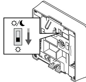
Optional: To activate tamper alarm for the thermostat, set the Disable timer switch to Comfort mode (⚙️) before registering the thermostat.
