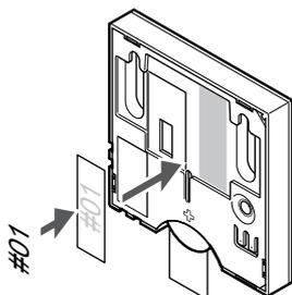
Label the thermostat, where suitable, with the channel numbers they are to control, for example, #02, #03. For a system with several room controllers, add the ID of each room controller, for example, 1.02, 1.03, 2.02, 2.03.
