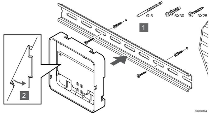
1. Fasten the DIN rail to the wall using the screws and wall plugs.
