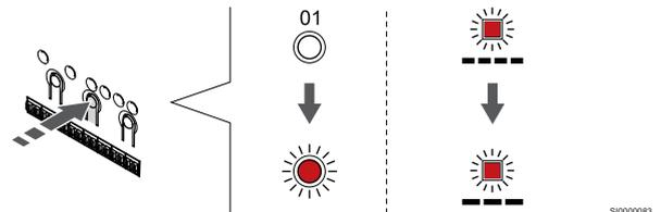
Press the **OK** button to enter system device registration mode (power LED). The power LED starts flashing according to the pattern long blink, short pause, long blink. Channel 1 starts flashing red.
