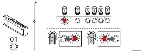
Use buttons < > to move the pointer (LED flashes red) to channel 1.
