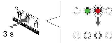
Press and hold the **OK** button on the room controller until the green LEDs turn off to end registration and return to run mode.
