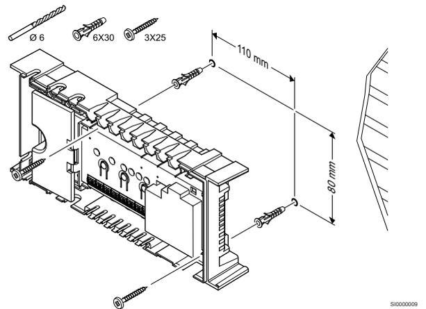
Attach the room controller to the wall using screws and wall plugs.
