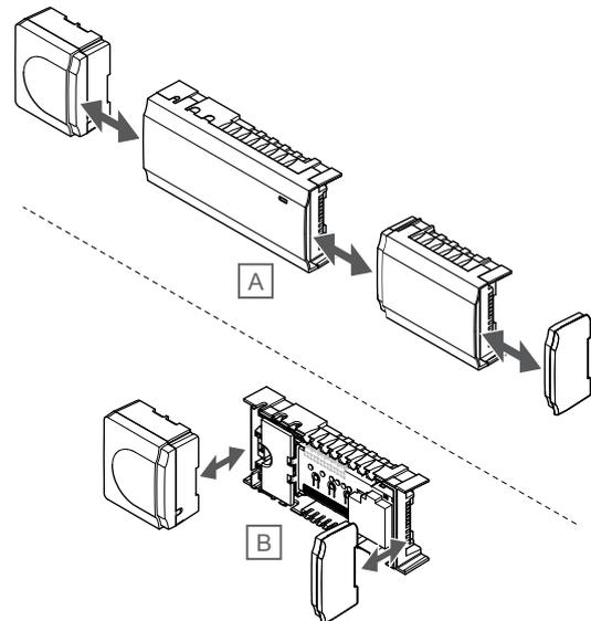
The components can either snap on or off without the need of removing the covers (A, recommended to do on a flat surface or on a DIN-rail), or by sliding them into place when the covers are removed (B).
