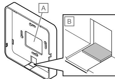
Route cables to the communication module using one of two cable entries.
