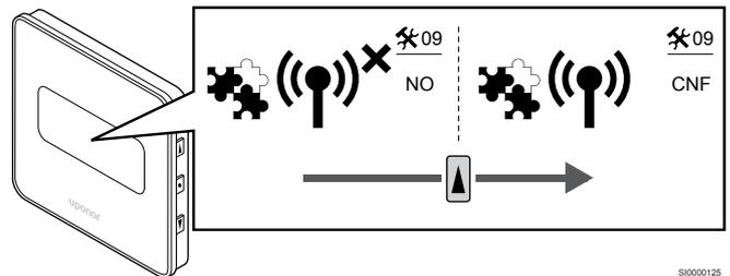
The connection indicator is shown in the thermostat display to show that the registration process begins.
