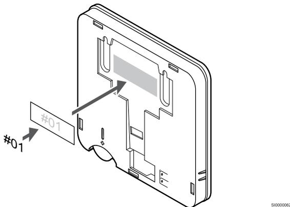
Label the thermostat, where suitable, with the channel numbers they are to control, for example, #02, #03. For a system with several room controllers, add the ID of each room controller, for example, 1.02, 1.03, 2.02, 2.03.
