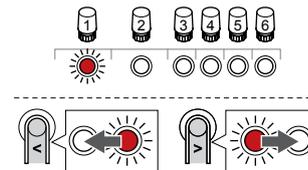
Use buttons < or > to move the pointer (LED flashes red) to the channel to unregister (solid green LED).
