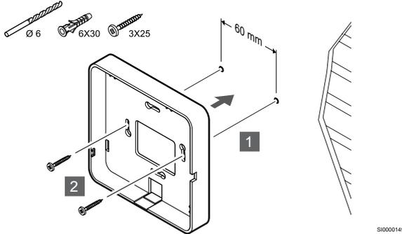
Attach the communication module back mount to the wall using the screws and wall plugs.
