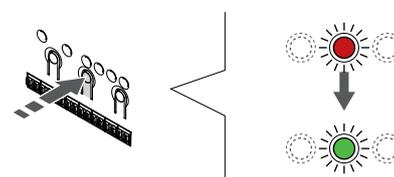
Press the **OK** button to select the channel for registration. The LED for the selected channel starts flashing green.
