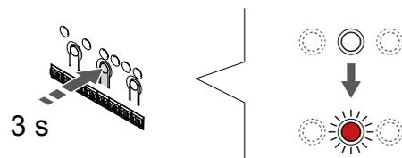
Press and hold the **OK** button on the room controller until the LED for the first unregistered channel flashes red. If all channels are registered to thermostats, the LED flashes red and green.
