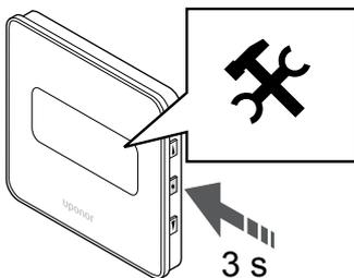
Press and hold the **OK** button for about 3 seconds. The settings icon and menu numbers is displayed in the top right corner of the display.
