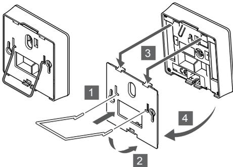
Attach the table stand to the thermostat using the wall bracket.
