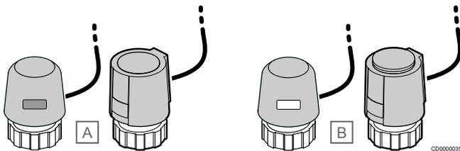
A Actuator has closed the valve – empty indicator
