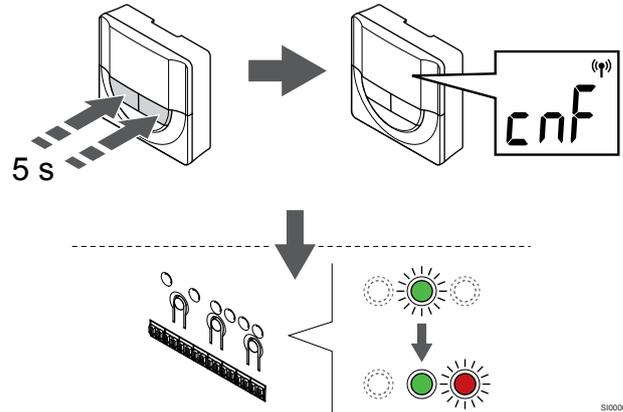
Press and hold both **-** and **+** buttons on the thermostat until the text **CnF** (configure) and a communication icon is displayed.
