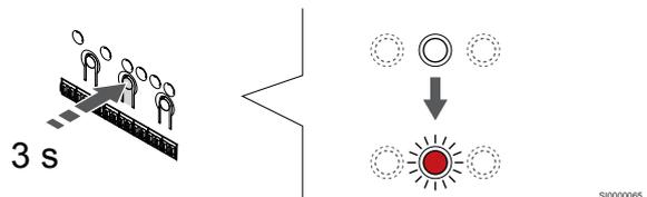
Press and hold the **OK** button on the room controller until the LED for the first unregistered channel flashes red. If all channels are registered to thermostats, the LED flashes red and green.
