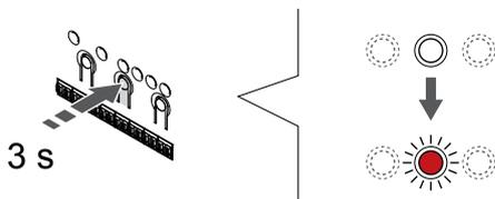
Press and hold the **OK** button on the room controller until the LED for channel 1 (or the first unregistered channel) flashes red.
