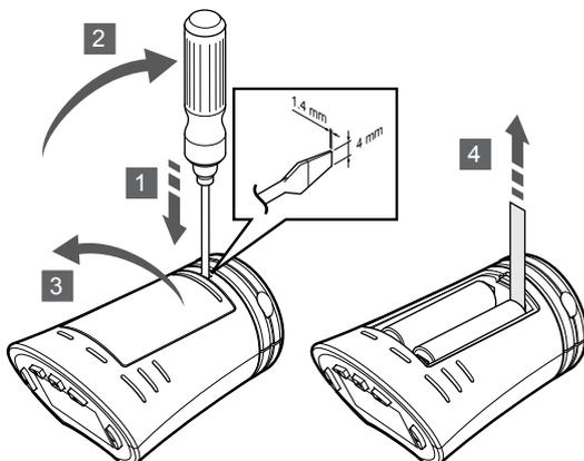
Remove the plastic transportation strips from the batteries to start the thermostatic head.
