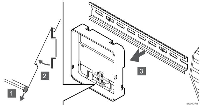
1. Use a screwdriver (or similar) and extend the springy plastic catcher from the communication module back mount.
