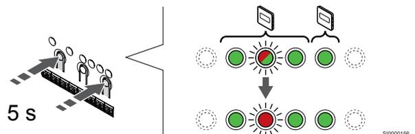
Press the < and > buttons simultaneously until the LED for the selected channel starts flashing red (about 5 seconds).
