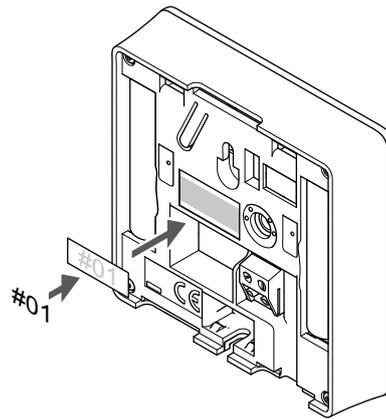
Label the thermostat, where suitable, with the channel numbers they are to control, for example, #02, #03. For a system with several room controllers, add the ID of each room controller, for example, 1.02, 1.03, 2.02, 2.03.
