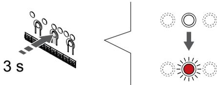
Press and hold the **OK** button on the room controller until the LED for channel 1 (or the first unregistered channel) flashes red.
