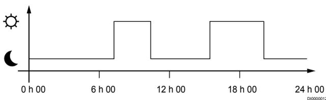
The diagram shows that the system delivers heating in comfort mode in the morning and afternoon, but the system enters ECO mode during night and in the middle of the day, when the house normally is empty.
