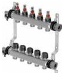
Uponor Vario S Flowmeter Manifold is a stainless steel manifold for use in radiant heating systems, where flow needs to be shown. The 3/4" Eurocone connectors allow for the connection of all Uponor pipe dimensions (Eurocone adapters page 76). Which makes this manifold universal for Uponor underfloor heating systems. Comes complete with fill and drain points, 1" swivel connectors and valve pins for actuator control. (Not suitable for 60°C+ systems).
