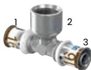
Made of plated DZR brass with size colour coded press stainless steel sleeve. Central BSP 'Rp' type female threaded adapter for screw connections to BS EN 10226-1.
