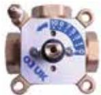
Made from DZR brass. Rotary shoe valve used to blend the system water to the required temperature.
