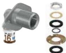
Twist proof connection for wall penetrations. Requires a 33mm hole. Made from plated DZR brass with size colour coded stainless steel press sleeve. BSP 'R' type male thread for screw connections to BS EN 10226-1. Fitting kit included.
