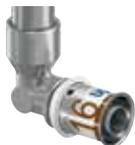
Body of the fitting made from plated DZR brass with size colour coded stainless steel press sleeve. BS EN 1057 plated copper pipe 15x1mm and 12x1mm. \*Not S-Press PLUS.
