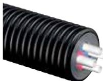
Ecoflex Quattro pipe PEX, 10 bar / 70°C DHW and 6 bar / 80°C LTHW. (Contains 2 x Thermo Pipes and 2 x Aqua Pipes).
