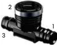
Made from engineered plastic (PPSU). Uponor Q&E Shrink-fit connections on both ends, with female BSP 'RP' type thread. For connections to BS EN 10226-1.
