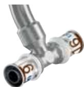
Body of the fitting made from plated DZR brass with size colour coded stainless steel press sleeve. BS EN 1057 plated copper pipe 15x1mm.
