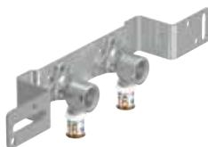
Mounted Aqua tap elbow assembly. Fittings made from plated DZR brass with size colour coded stainless steel press sleeve. BSP 'Rp' type female threaded screw connections to BS EN 10226-1.
