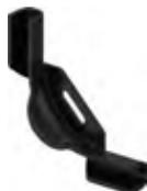
Bend supports are used where the PEX pipe is returning up from the floor towards the manifold. This creates a stable 90° bend making it easier for the installer to connect to the manifold.
