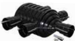
For sealing connections of single main lines (flow and return) to twin outlet lines in the trench. Comprises of insulating half-shells, stainless steel screws, plastic dowels and sealant. Only to be used with Uponor rubber end caps.
