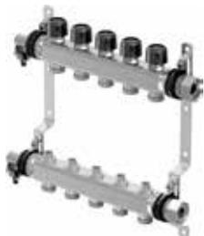
Uponor Vario S Lockshield Manifold is a stainless steel manifold for use in radiant heating systems, where balancing is done by a hex key. The 3/4 Eurocone connectors allow for the connection of all Uponor pipe dimensions (Eurocone adapters page 76). The manifold is universal for all Uponor underfloor heating systems. Comes complete with fill and drain points, 1" swivel connectors and valve pins for actuator control. (Suitable for radiator systems).
