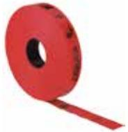
To mark the position of buried pipes. Red, tear-proof plastic tape imprinted with 'Uponor' and symbols for trench identification.
