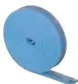
For use on Minitec system, to reduce thermal bridging. Made of polyethylene with self adhesive backing and PE skirt providing tight seal between edge strip and insulation. Thermal resistance 0.22m<sup>2</sup>K/W. Supplied in 20m rolls, 80x8mm HxD.
