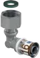
Made from plated DZR brass with size colour coded stainless steel press sleeve. BSP swivel nut connection with flat sealing washer.
