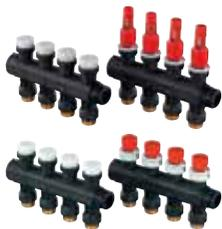
Made of a reinforced glass fibre polyamide body. Its primary use is for underfloor heating and cooling applications as it is less prone to corrosion and condensation. It is available in modules of 1, 3, 4 and 6 loops with corresponding connection sets sold separately. The secondary connectors allow the connection of all Uponor pipe dimensions (Eurocone adapters page 76).
