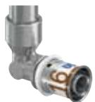
Body of the fitting made from plated DZR brass with size colour coded stainless steel press sleeve. BS EN 1057 copper pipe 15x1mm and 22x1mm. \*Not S-Press PLUS.
