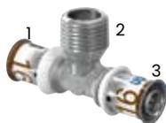
Made of plated DZR brass with size colour coded press stainless steel sleeve. Central BSP 'R' type male threaded adapter for screw connections to BS EN 10226-1.
