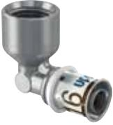
Made from plated DZR brass with size colour coded stainless steel press sleeve. BSP 'Rp' type female threaded adapter for screw connections to BS EN 10226-1.
