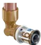
Body of the fitting made from DZR brass with size colour coded stainless steel press sleeve. BS EN 1057 copper pipe 15x1mm.
