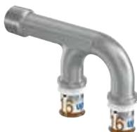
Made from plated DZR brass with size colour coded stainless steel press sleeve. BSP 'R' type male thread connection. For use in 'serial' or 'loop' type installations.
