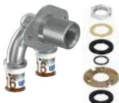
Twist proof connection for wall penetrations. Requires a 33mm hole. Made from plated DZR brass with size colour coded stainless steel press sleeve. BSP 'R' type male thread for screw connections to BS EN 10226-1. For use in 'serial' or 'loop' installations. Fitting kit included.
