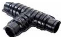
For sealing T-connections of Single, Twin and Quattro pipes in the trench. Comprises of insulating half-shells, stainless steel bolts and sealant. Only to be used with Uponor rubber end caps.
