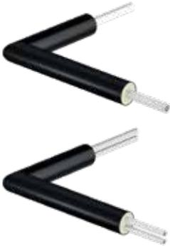
Pre-insulated PE-Xa pipe 90deg elbows with single or twin pipes. Max. load 6 bar /95c. PUR Foam insulation with PE casing
