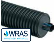
Ecoflex single pipe PE-HD, max. 16 bar / 20°C, complete with frost protection cable. For chilled water and potable water. **Use Plasson coupling or Wipex 6 bar coupling. Please add 1 metre of extra pipe to allow for electrical connection.**
