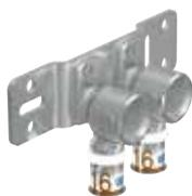
Mounted Aqua tap elbow assembly. Fittings made from plated DZR brass with size colour coded stainless steel press sleeve. BSP 'Rp' type female threaded screw connections to BS EN 10226-1.
