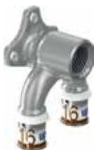
Made from plated DZR brass with size colour coded stainless steel press sleeve. BSP 'Rp' type female thread connection. For use in 'serial' or 'loop' type installations. Mounting brackets and fixings on page 43.
