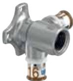
Made of plated DZR brass with size colour coded stainless steel press sleeve. BSP 'Rp' type female threaded connection – long. \*Not S-Press PLUS.
