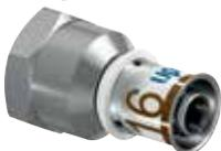
Made of plated DZR brass with size colour coded stainless steel press sleeve. BSP 'Rp' type female threaded adapter for screw connection to BS EN 10226-1. \*Not S-Press PLUS.
