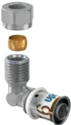
Made from plated DZR brass with size colour coded stainless steel press sleeve. Compression type connection to 10mm copper pipe.
