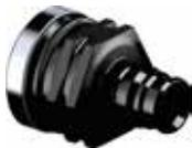
Uponor Q&E Shrink-fit connection on one end, with BSP 'Rp' type female-threaded adapter for screw connections to BS EN 10226-1.
