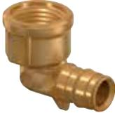
Uponor Q&E Shrink-fit connection on one end, with BSP 'RP' type female-threaded adapter for screw connections to BS EN 10226-1.
