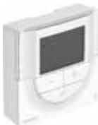
A wireless digital programmable thermostat with Rh sensor and large backlit display. It measures and displays the room temperature and Rh, and subsequently transmits the values to the wireless controller.
