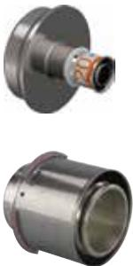
Made of tin plated brass with stainless steel press sleeve. For connection of MLC to RS2/RS3 Bodies. **Note: All RS-Press Adapters must only be pressed using the approved Uponor UP75 or UP110 (1083612) tools.** \*S-Press PLUS connection.
