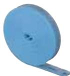
For use on Siccus Mini system, to reduce thermal bridging. Made of polyethylene with self adhesive backing and PE skirt providing tight seal between edge strip and insulation. Thermal resistance 0.22m<sup>2</sup>K/W.
