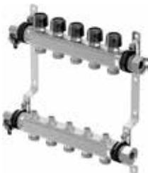
Stainless steel flow and return manifolds for heating. Comes complete with mounting brackets. Lockshield valves supplied. Actuators can be added if required page 86 or page 87. Primary connections are 1" BSP threads, outlet connections are 3/4" Eurocone (sold separately).
