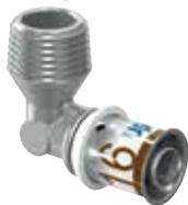
Made from plated DZR brass with size colour coded stainless steel press sleeve. BSP 'R' type male threaded adapter for screw connections to BS EN 10226-1.
