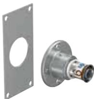
Twist proof connection for wall penetrations. Requires a 33mm hole. Made from plated DZR brass with size colour coded stainless steel press sleeve.
