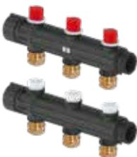
Magna Manifold range of 1, 2 or 3 port units for connection with additional segments and basic kit. Supply-segment with control valves for pre-adjustment, return-segment with thermostat upper section including cap for locking. Uponor actuator can be mounted directly on the return. Heating loop connection for PE-Xa pipe 25x2.3 with compression adapter.
