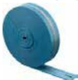
For use on solid screed floors as perimeter wall insulation, to reduce thermal bridging. Made of polyethylene with self adhesive backing. Thermal resistance 0.22m<sup>2</sup>K/W. Supplied in 50m rolls, 150mm (H) x10mm (D).
