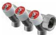
Supplied as a single manifold. Made of plated brass,  $\frac{3}{4}$ " or 1" MT x FT connections with  $\frac{1}{2}$ " or  $\frac{3}{4}$ " MT outlets. Valves allow each circuit to be isolated. Delivered with loop labelling discs. Order adapters separately for connection to Uponor pipe (MLC/SAC/Q&E). Manifolds can be joined to make the required number of ports. 5 bar maximum operating pressure.
