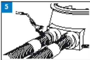
Preheat the area that is left under the shrink sleeve using a soft gas flame. Remove the protective paper from the sleeve and place the sleeve around the joint.
