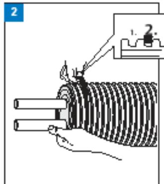
Install the rubber seal in the second groove.
