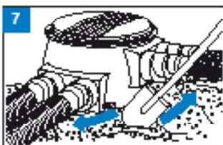
Close the chamber lid, but tighten the bolts only after the pipeline has been pressure tested. Begin filling the trench by pushing sand underneath the joints.
