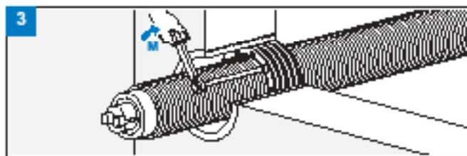
During final assembly, successively tighten up each nut with torque-wrench clockwise until the maximum torque  $M_{max}$  is reached. Tighten the nuts several times. Repeat the procedure after two hours.
