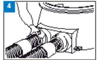
Roughen up the surface of the jacket and the chamber joint with sand paper around the shrink sleeve. Wipe the joint area clean.
