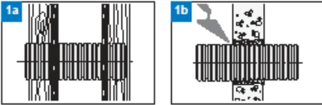
Place the feed-through sleeve in the structure where the pipe element will be placed and cast into place at a later stage. Please note that at least 10cm of the sleeve should be left outside the cast.
