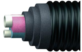
**Uponor Quattro** pre-insulated quad-pipe PE-X, max. 6 bar / 95°C, Heating and/or max. 10 bar / 95°C / warm water
