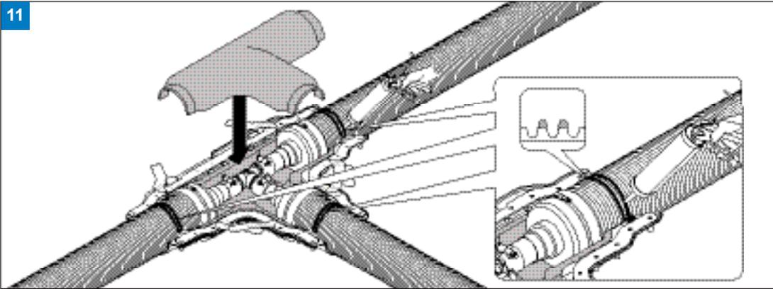
Position upper foam half-shell over joint area. Apply sealant to two corrugations where pipe meets spacer piece.
