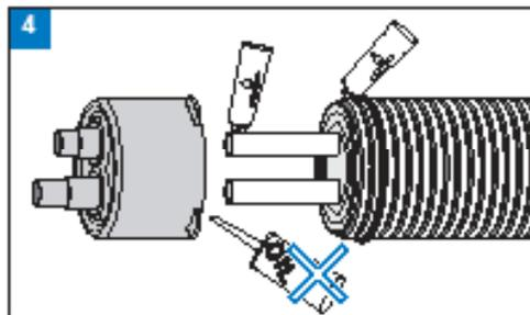
Install the end cap over the end of the pipe using lubricant. A non oil-based lubricant can assist.
