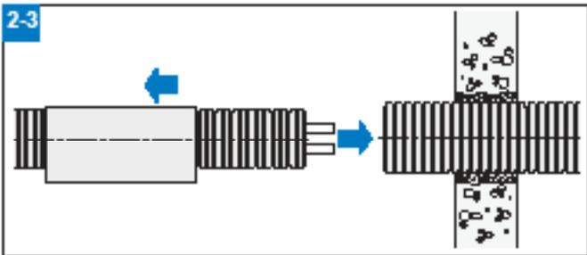
Install the shrink sleeve on top of the pipe element. Push the pipe element through the feed-through sleeve.
