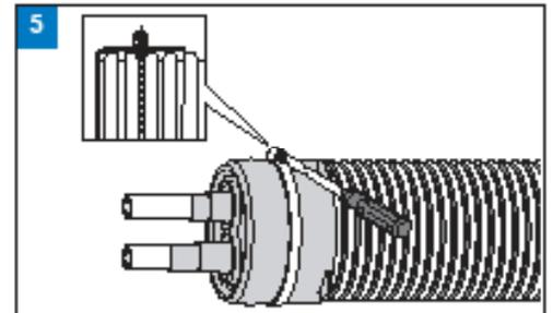
Position the jubilee clip over the seal and tighten.
