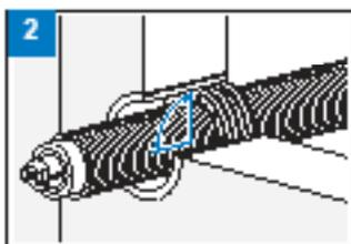
Install Uponor PWP wall seal pipe at right angles to Uponor pipe
