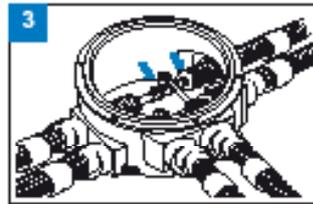
Push the pipes into the chamber. Fasten the rubber end caps on the jacket pipe using jubilee clips. Join the pipes and tighten the couplings.
