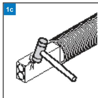
1c Using blunt tools break away the insulation to reveal the pipe(s). Been careful not to damage the pipe.
