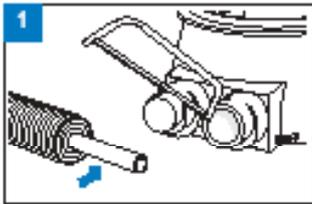
Cut open branches of the chamber according to the required pipe size. Peel off enough of the jacket pipe and insulation to make the joint, 10-20 cm depending on the pipe size.
