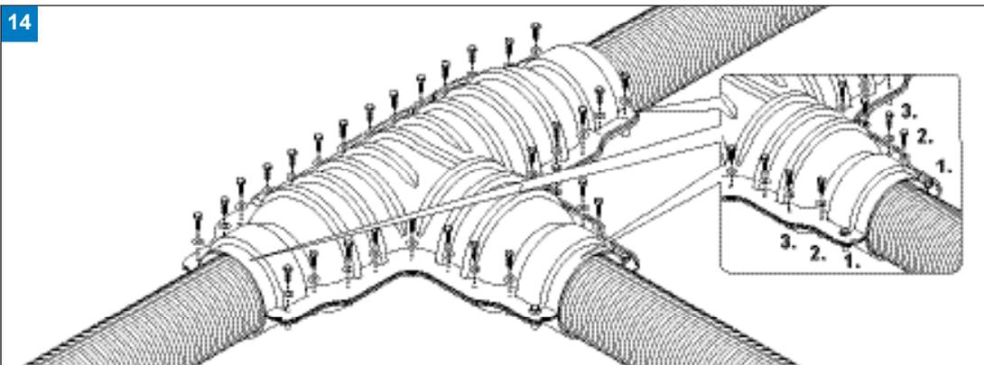
Complete assembly of insulation set using bolts provided.
