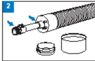
Put the end caps and their seals in place at the ends of the pipes. Mount the connectors to the ends of the flow pipes. Slide the shrink sleeves onto the pipes.
