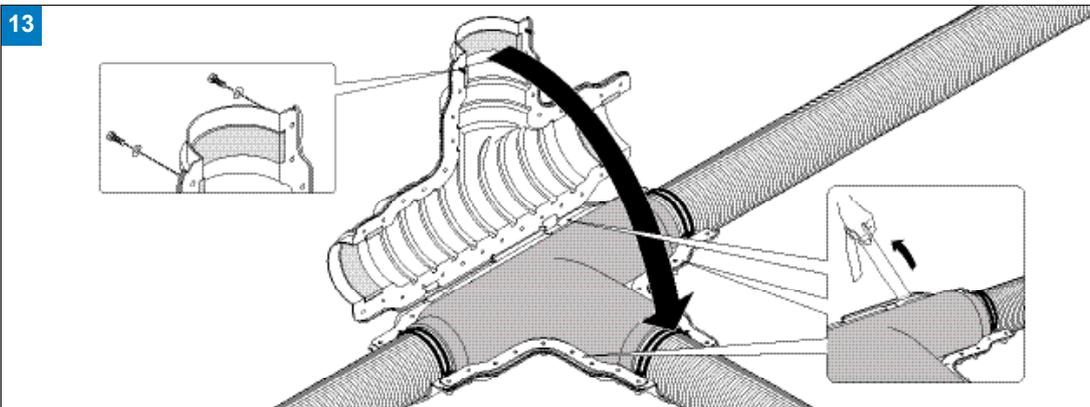
Fully release adhesive strips and position top half of casing over joint area.
