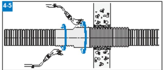
Place the shrink sleeve centrally in the joint between the sleeve pipe and the pipe element and remove any paper that may be left inside the shrink sleeve.
