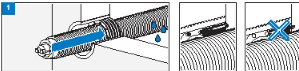
Insert the PWP wall seal as far as the water side (outside) - nuts face the cellar side
