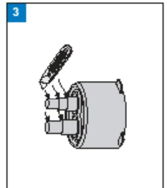
Open outlets on the rubber end cap according to the flow pipe size.
