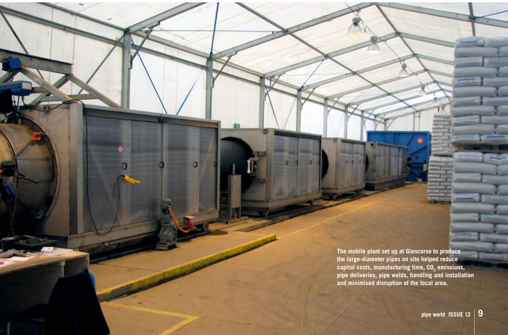
The mobile plant set up at Glencorse to produce the large-diameter pipes on site helped reduce capital costs, manufacturing time, CO<sub>2</sub> emissions, pipe deliveries, pipe welds, handling and installation and minimised disruption of the local area.
