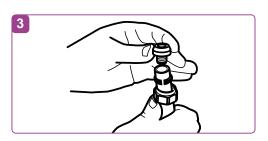
3. Installation of the union nut and locking ring First push the union nut and then the locking ring onto the end of pipe.
