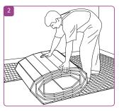
Lay the insulation roll length ways in the room and by matching the pre-printed grid
